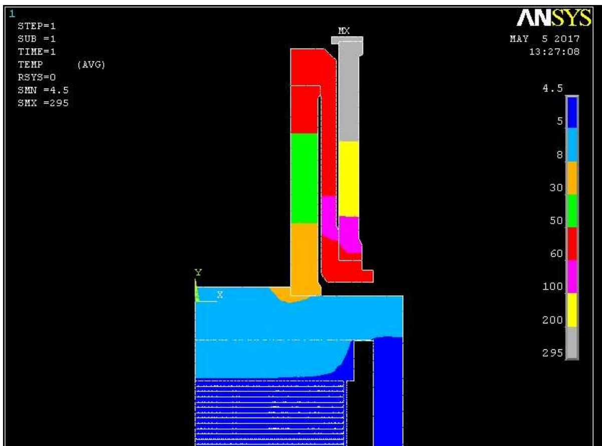
Fig. 22. Temperature distribution in the support struts at bulk temperature of 4.5 K and the heat transfer coefficient of 1 kW/(m 2 *K).
