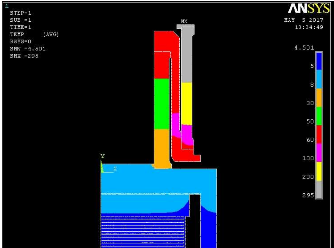
Fig. 23. Temperature distribution in the support struts at bulk temperature of 4.5 K and the heat transfer coefficient of 30 \text{ W}/(\text{m}^2 \cdot \text{K}) .
