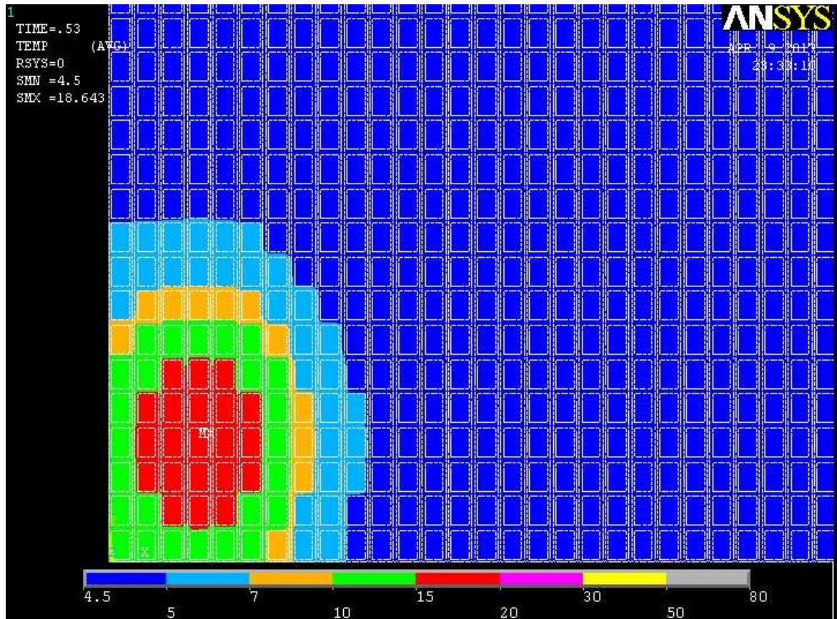
Fig. 26. Normal zone propagation in the winding in 2D calculations. Here time after start of the quench is 0.53 s, the quenched wire is in the center of the red zone and its maximal temperature is 18.6 K.
