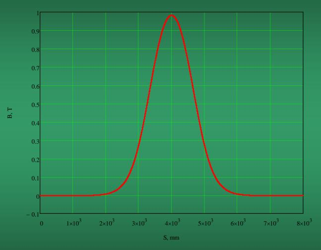
The integral from the target along the central line is 0.886 T\*m in the length of 1 m.
