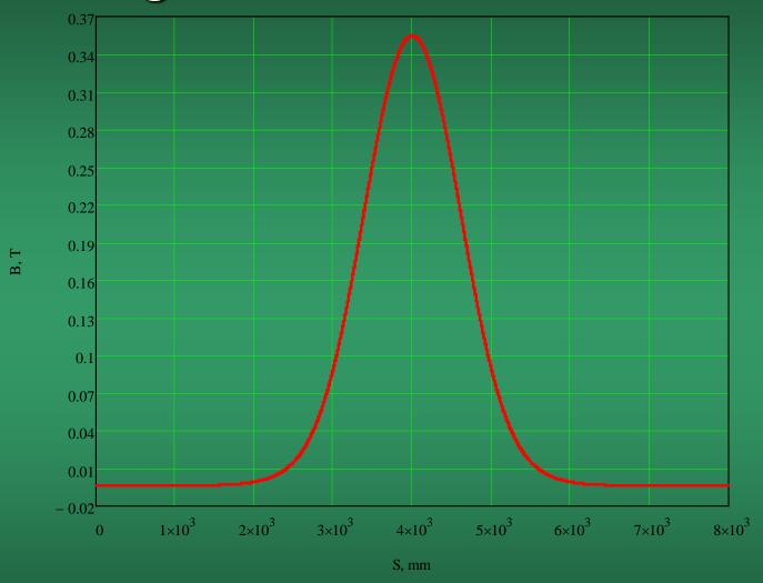
Magnetic field distribution at horizontal shift on 900 mm, vertical position is 0 mm from the center
