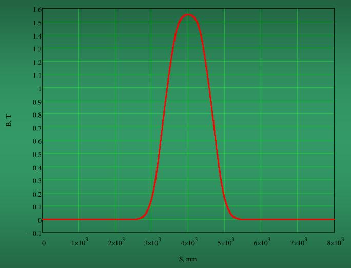
Magnetic field distribution at vertical shift on 450 mm, horizontal position is 0 mm.
