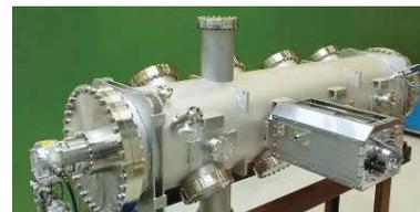
Prototype stochastic cooling tank at GSI
