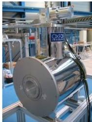
X-ray optics, channel-cut crystals
