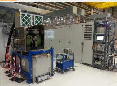
FOS debuncher cavity SAT ongoing.
