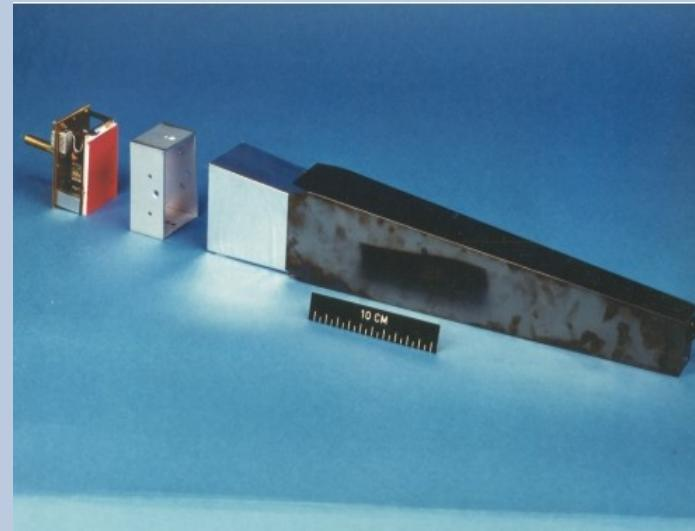
new designed readout based on APDs
