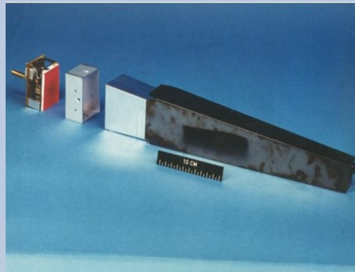
new designed readout based on APDs
