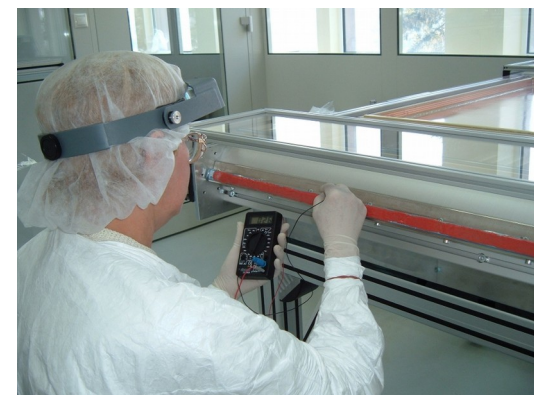
Checks of electrical connections of multiwire electrodes
