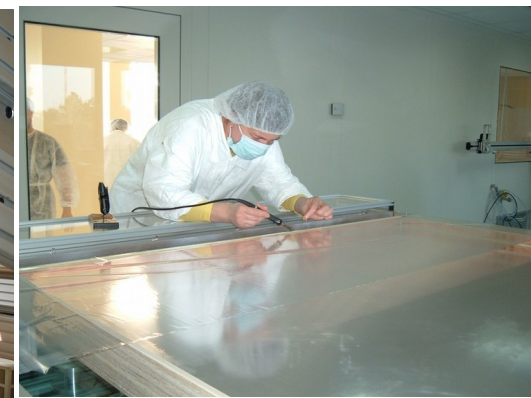
Soldering of the electrical connections of the multiwire electrodes
