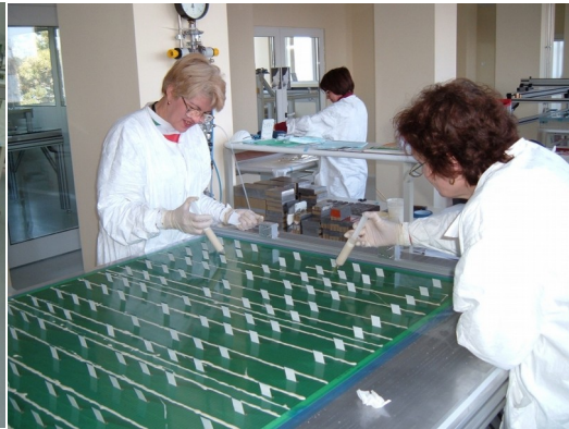
Pad plane assembling on the vacuum table
