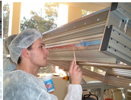
Multiwire electrodes winding using winding machine
