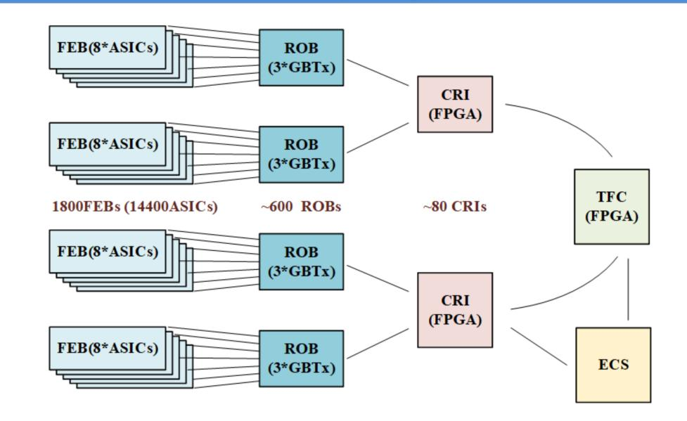
Hierarchy of the readout tree of the STS subsystem
