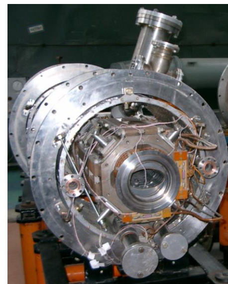
Nuclotron quadrupole inside cryostat
