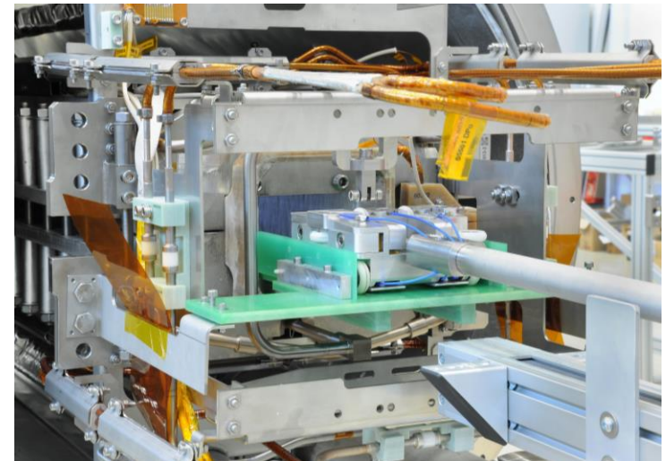
1 carriage, 2 capacitive sensors, 3 wheels, 4 holder for spherically mounted retroreflectors.
