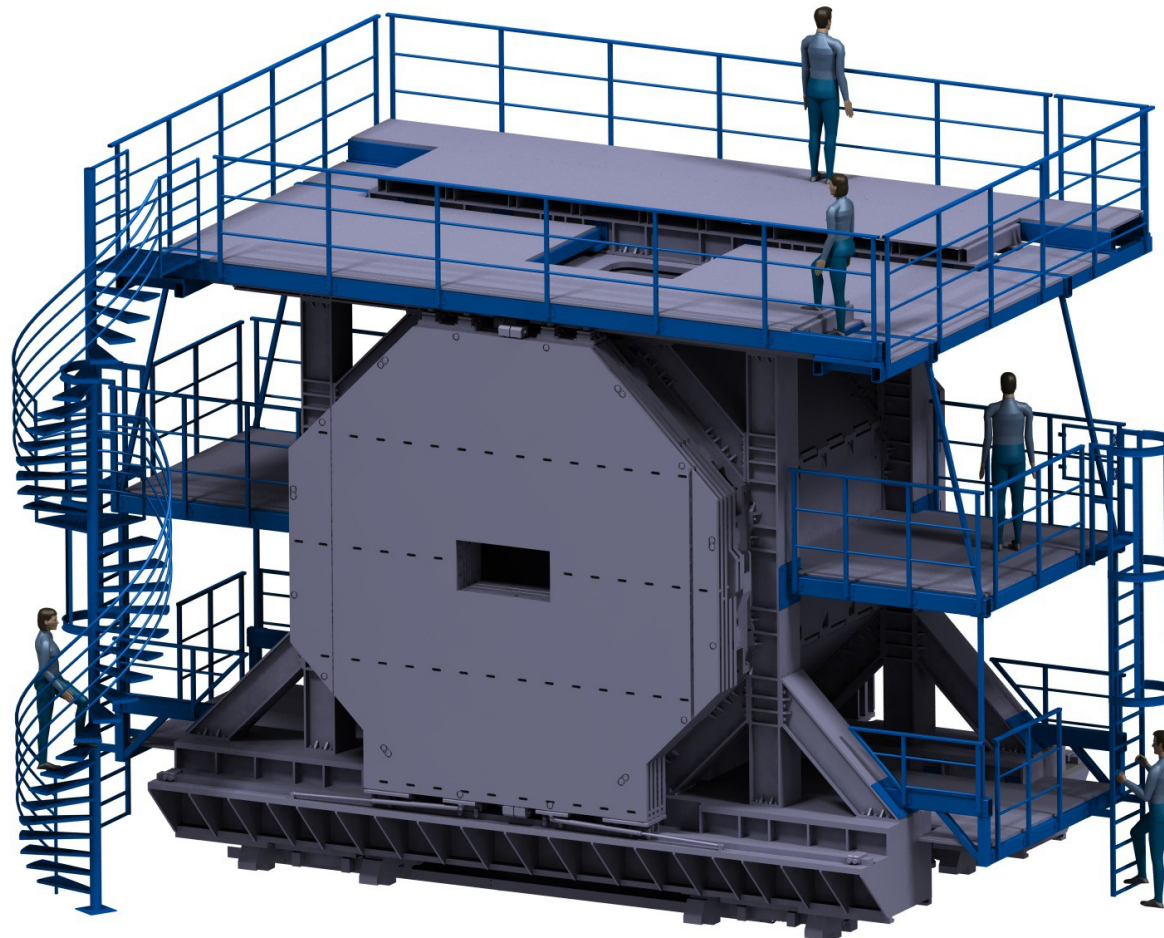
Solenoid with rack supports and top platform
