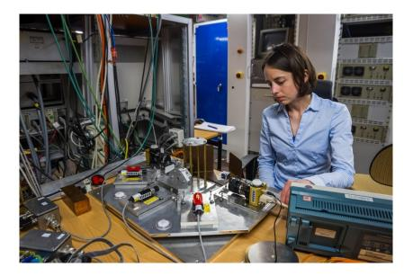
Installation of the detection module at the old PTR chamber.
