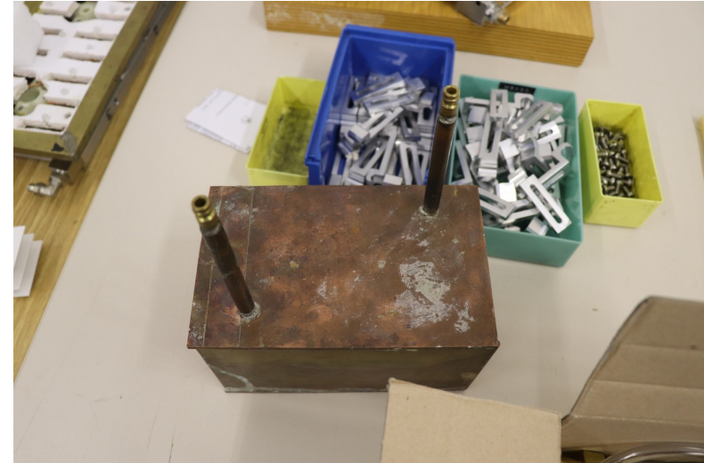
Heat exchanger for pressurized air
