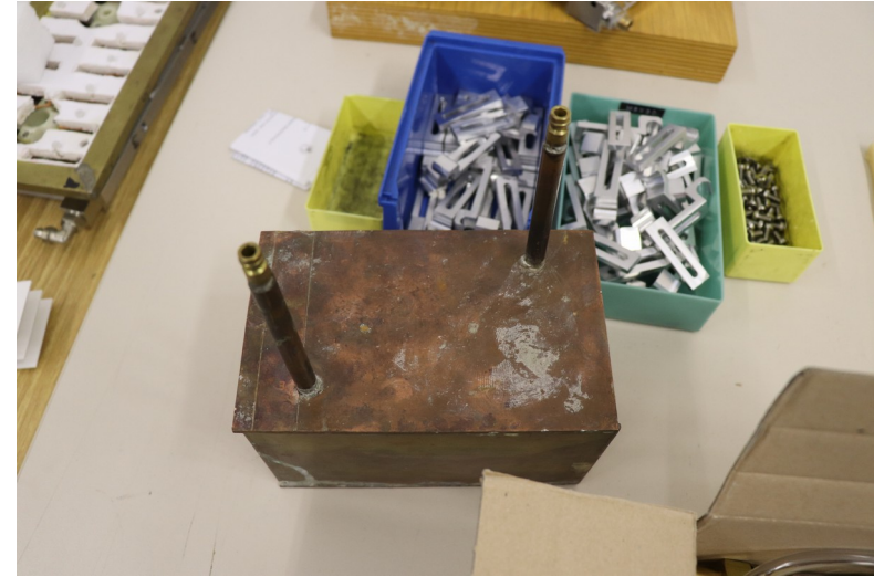
Heat exchanger for pressurized air
