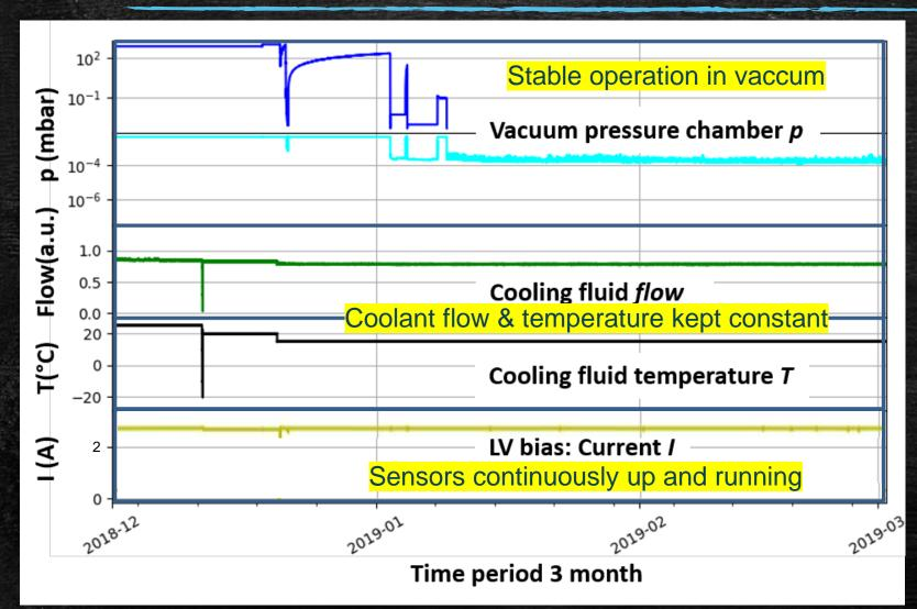
Plot showing a three month period of continuous prototype operation.
