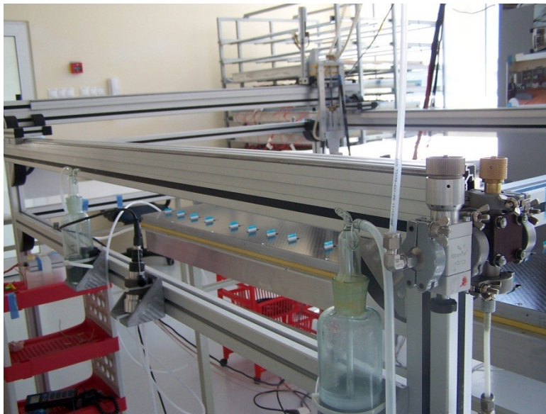
Gas leak rate test
