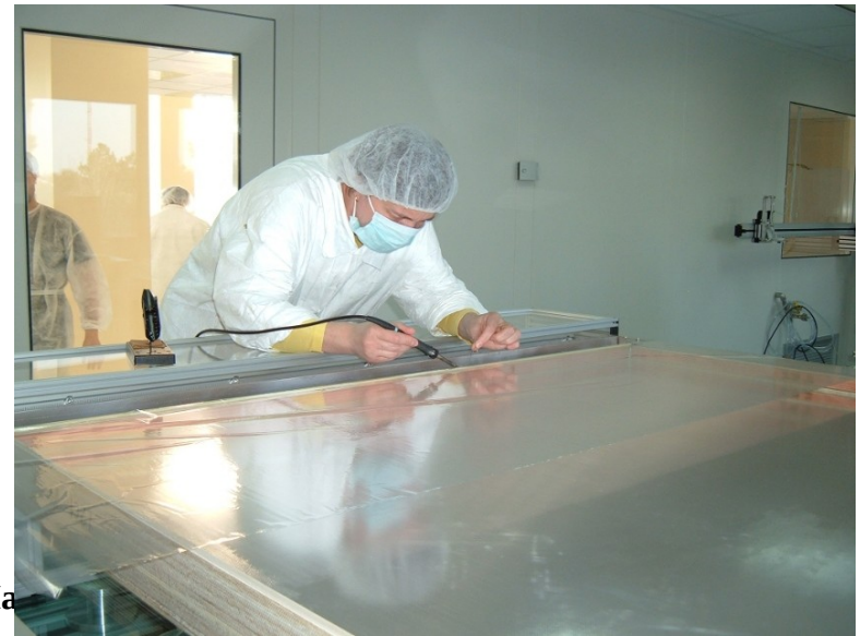
Soldering of the electrical connections of the multiwire electrodes in 10000 particles/ft 3 room
