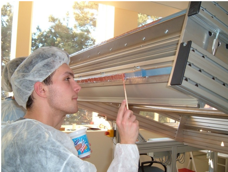
Multiwire electrodes winding using winding machine
