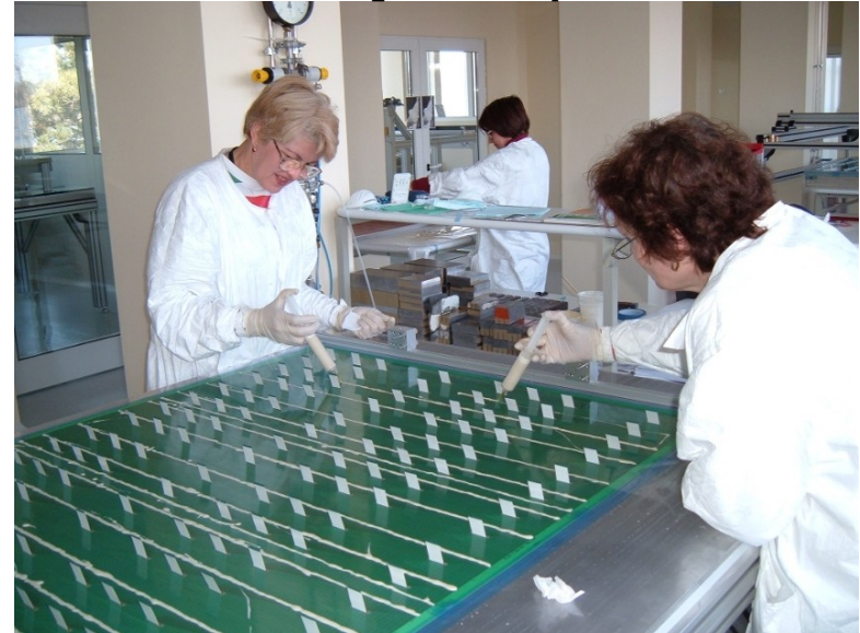
Soldering of the electrical connections of the multiwire electrodes in 10000 particles/ft 3 room
