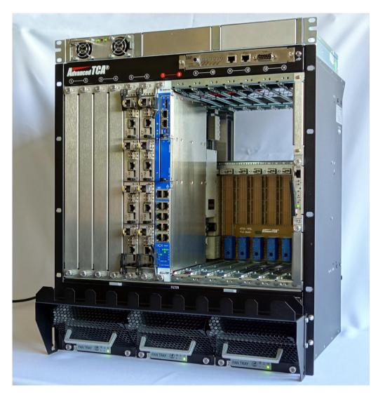
Two fully equipped Compute Nodes, one backplane GbE switch
