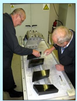
Precise gluing in packs of five units using devices, Special hardening technology in oven.
