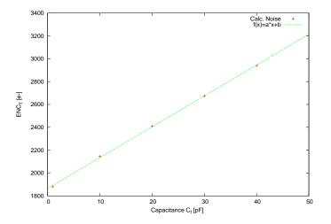
• Small capacitance for small signals  $\Rightarrow$  better SNR
