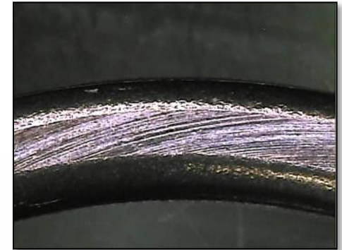
Poor Flange Finish: Radial Marks
