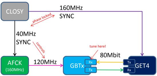
Only one point to tune! All other relationships are given by cable delays and fix for a given setup
