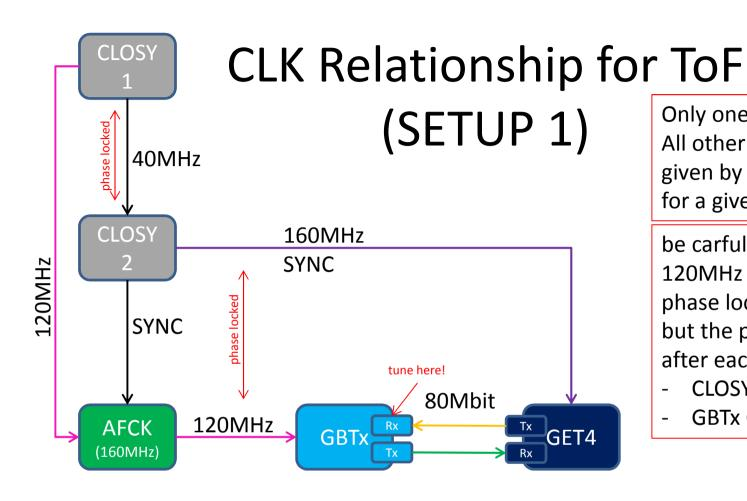
Only one point to tune! All other relationships are given by cable delays and fix for a given setup
