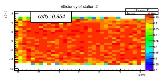
Tracking allows for spacial differential performance analysis Example for Tsinghua's Type a RPC
