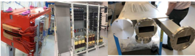
Bipolar dipole magnet, power converter and chamber for the connection of beam transport line to SIS100 ready for installation
