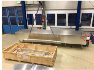
Drying Oven (5 m x 1.5 m x 1.5m /~5000€)
