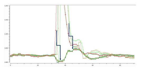
Crosstalk is not observed at processing crate and samtec cable
