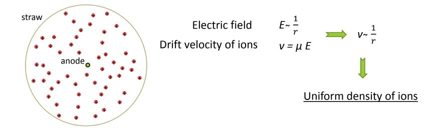
$$V = \int_{a}^{b} E_{w}(r) dr + \int_{a}^{b} E_{s}(r) dr \qquad \underline{E_{w}} \text{ (and gas gain) reduced if the 2nd integral > 0}$$
