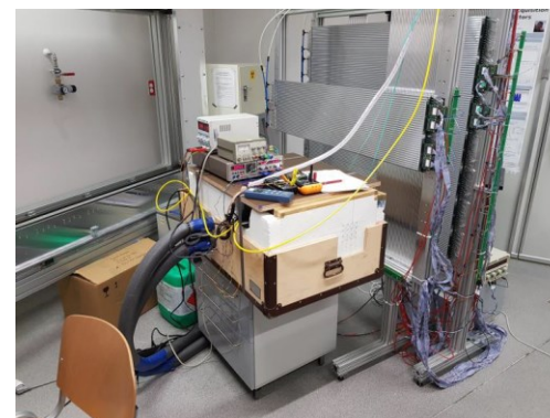
Straw (256ch, TRB3) & EMC (3x3 crystals, ADC) & PANDA-DAQ (3 CN) test setup in Krakow
