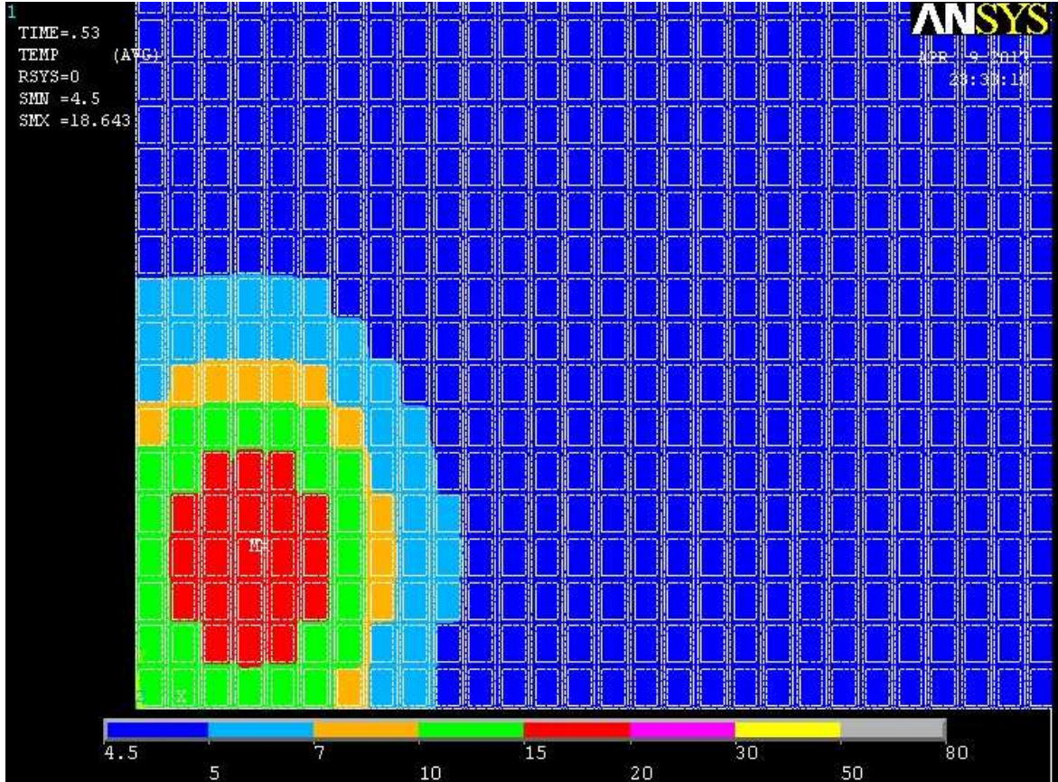
Fig. 40. Normal zone propagation in the winding in 2D calculations. Here time after start of the quench is 0.53 s, the quenched wire is in the center of the red zone and its maximal temperature is 18.6 K.
