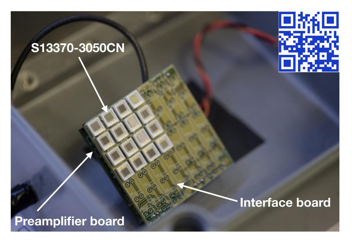
S13370-3050CN = VUV4 MPPC family manufactured by Hamamatsu
