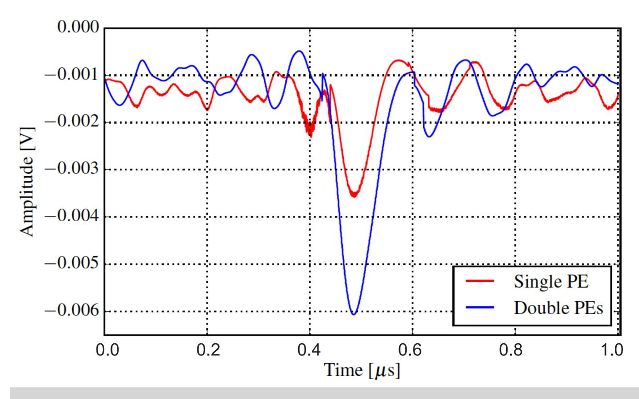
Typical waveforms corresponding to a single photon and to 2 photons taken at 175 K, 2 V of over-voltage (50  $\Omega$  termination).
