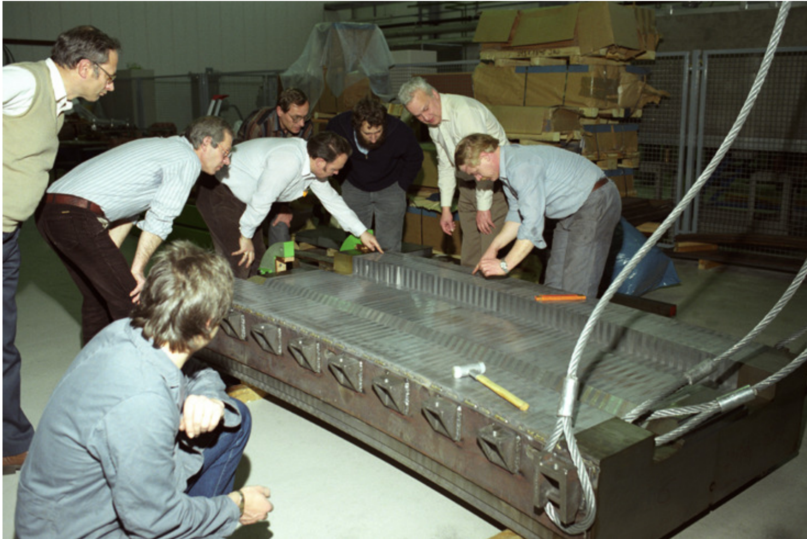
Preparing the next (whatever) step for an extension of the GSI facility: Prototype magnet for a 18Tm synchrotron (1983)
