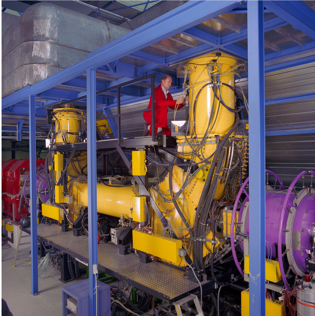
ESR Electron cooler, operating in a wide ion beam energy range, 3 – 490 MeV/u
