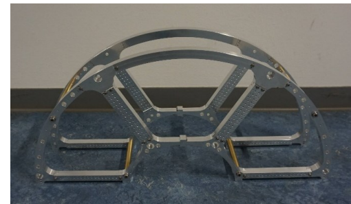
STT FE-volume for cooling tests, walls will be covered
