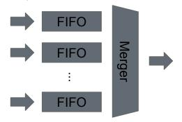
Maximum stream bandwidth is equal to the number of samples going through the pipeline in parallel when all samples are valid (no empty samples).
