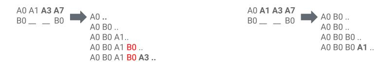
Merger outputting a sample on each clock cycle
