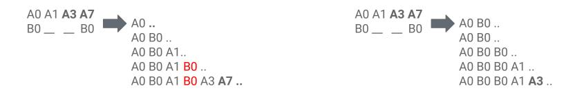
Merger outputting a sample on each clock cycle
