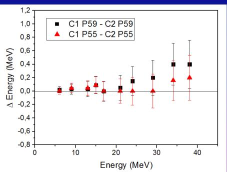
The two crystals have the same response (within the error bars) for high energy  $\gamma$ -rays
