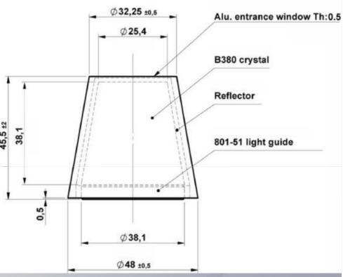
Truncated conical crystals 1x1.5x1.5" LaBr<sub>3</sub>(Ce)
