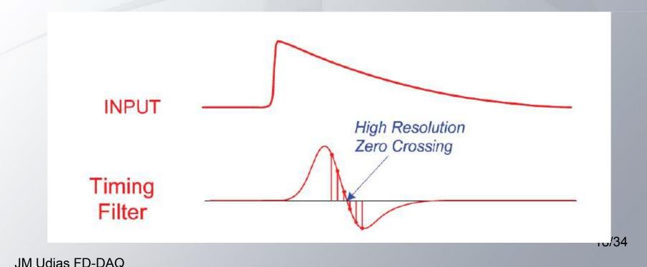
2.) A simple procedure, use crossing of *relative* thresholds for time stamping, instead of absolute ones: provides independence on the amplitude of the pulse. Easier implemented in digital world than in analog one
