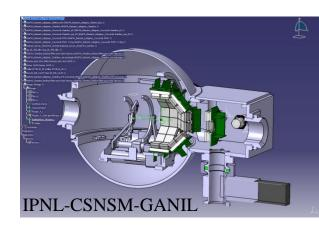
The final mechanical design of NEDA + NWALL foresees the use of 54 self produced NEDA detectors at forward angles and 14 NWALL detectors at around 90 degrees
