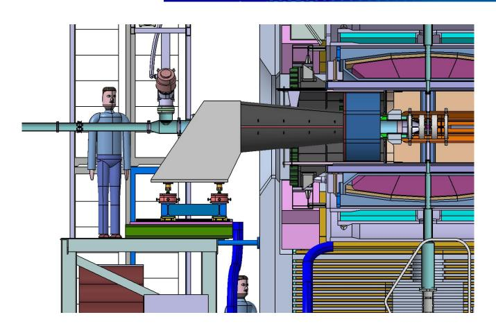
Lever arm concept with horizontal cone support
