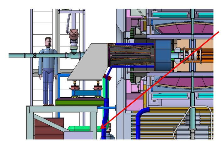
Then cables go down and under the Aux-Platform to the bottom left downstrea m rack
