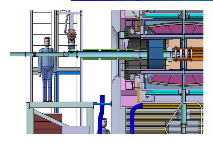
EMC BWEC distance from the target: **560mm**
