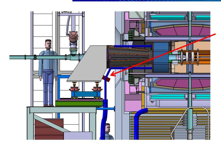
Patch Panel attached to the movable trolley
