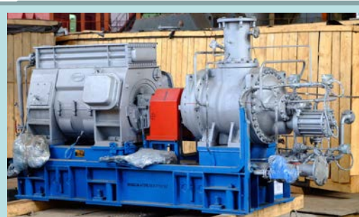
Helium screw compressors “Kaskad-110/30”
