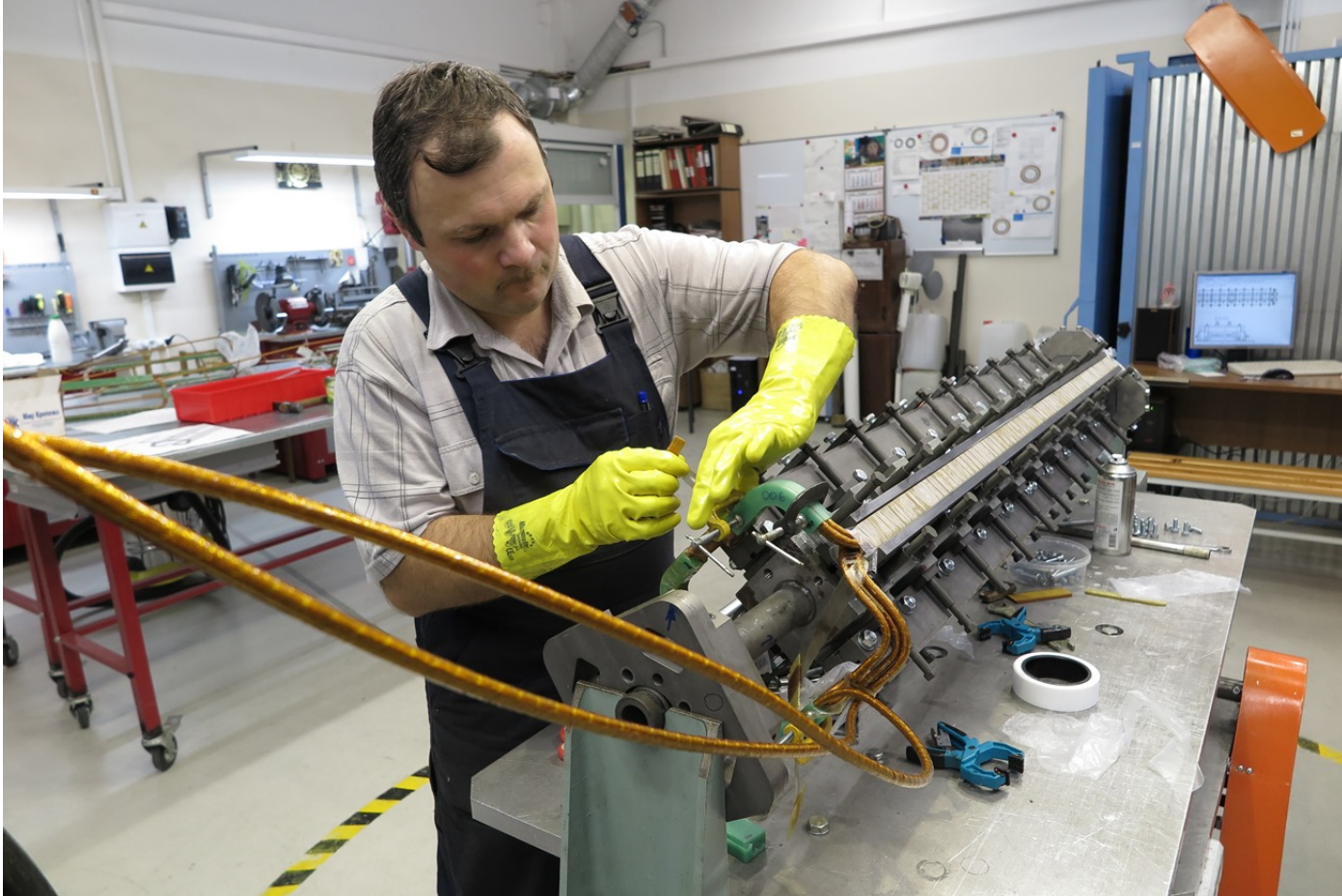
Manufacturing of the SIS 100 quadrupole coil
