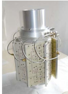
Ring slot-coupler RF structure (design FZJ)
