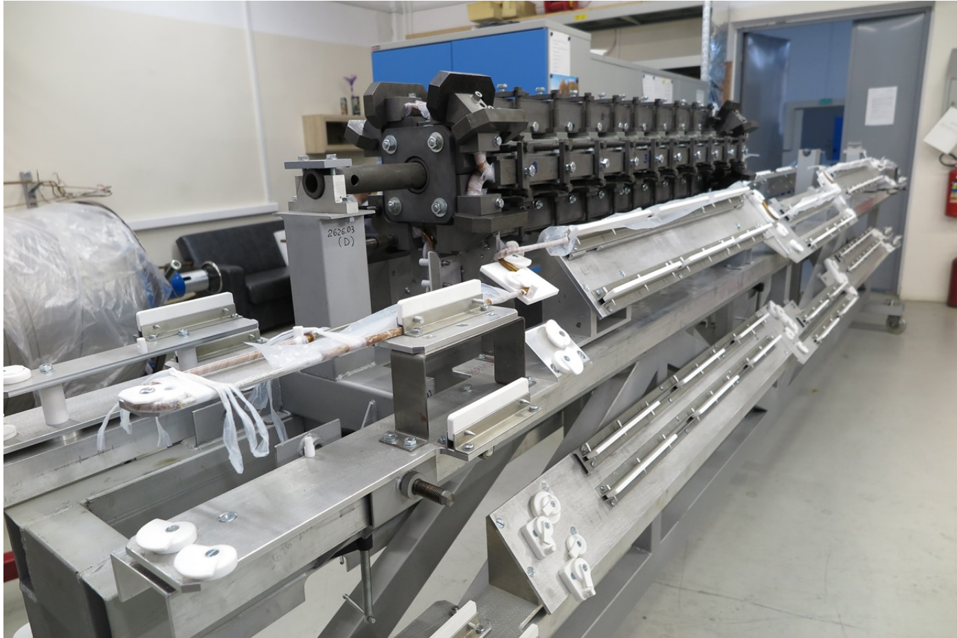
The SIS 100 quadrupole coil prepared to heat treatment in oven
