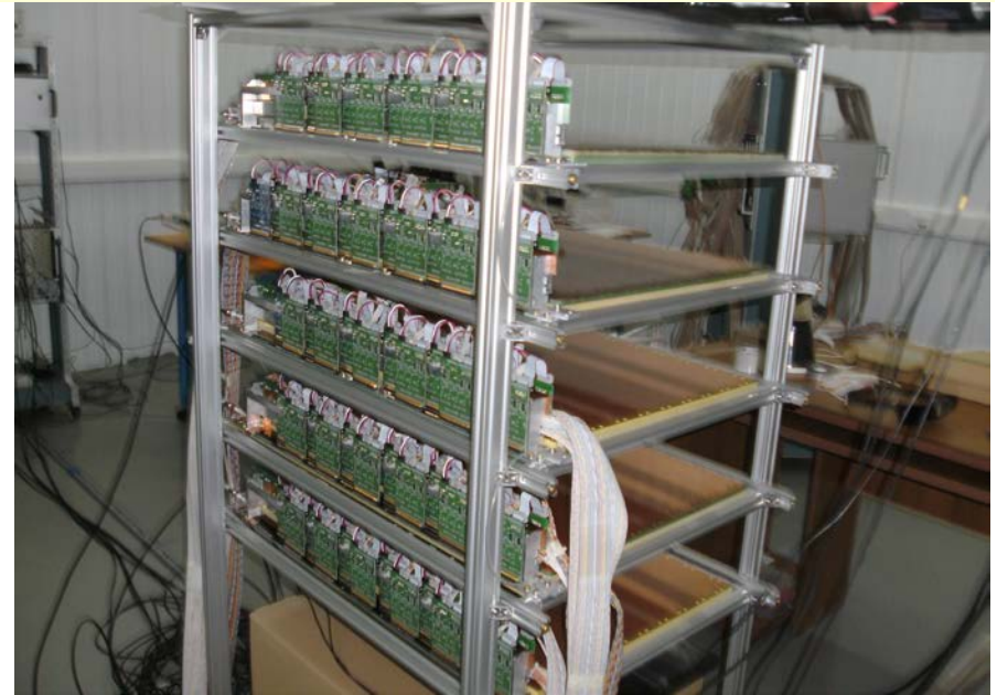
Set of 5 GEM detectors 66 x 41 cm 2 prepared for cosmic tests, June 2016
