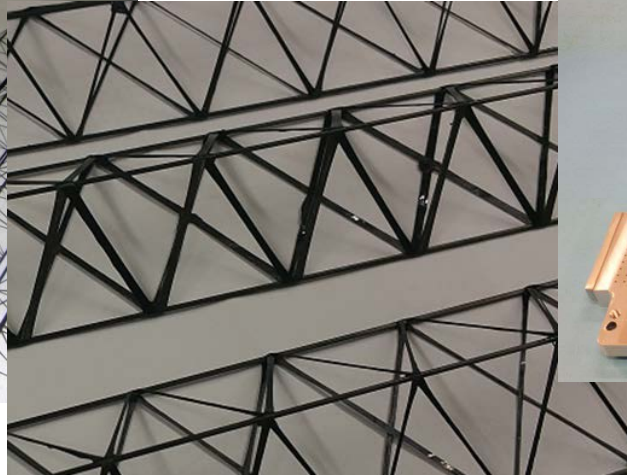
pre-series carbon-fiber ladders made in industry, GSI
