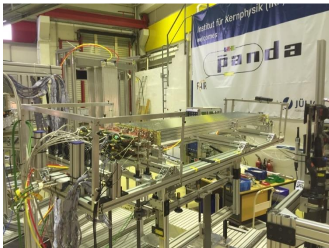
In-beam position of straw setup with FE-ASIC boards (beam from the right)
