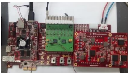
Testboard with ADC (LTM9011-14) and FPGA readout (ZEA- 2/FZJ)
