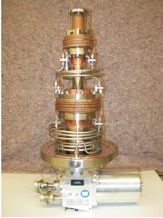
Figure 4.12: The complete mounted prototype of the PANDA cluster beam production head with the nozzle on the very top. Clearly visible are the gas pipes which are connected to the coldhead. The cables are used for the electric connection of the nozzle heating system as well as for the silicon diodes used for the gas temperature measurement.
