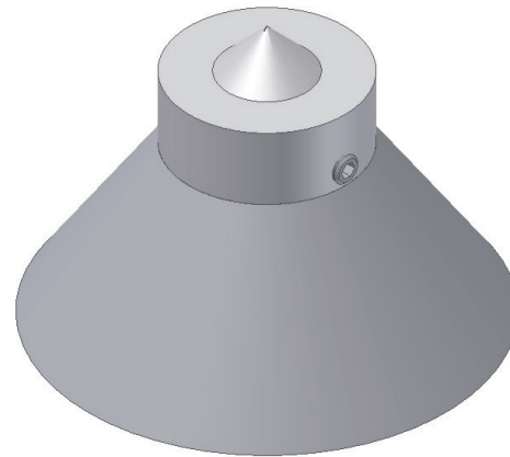
Figure 4.14: CAD-drawing of a slit collimator produced by a special laser cut process.
