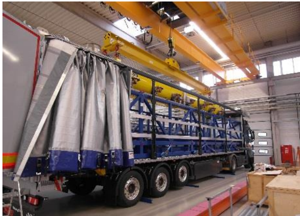
■ Unloading of the cryomodule after transport
