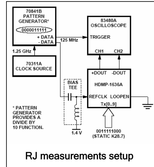
Jitter measurement of full chain is needed
