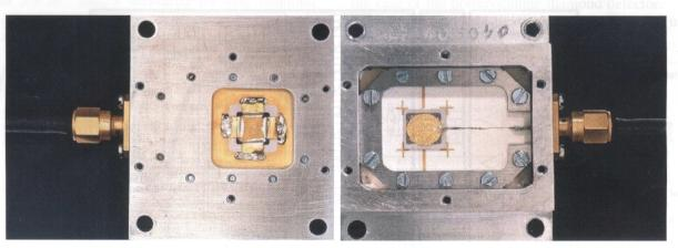
Fig. 1. Each single-channel of a CVD-diamond HI detector is connected via a  $50-\Omega$  microstrip line to the amplifier. The fully metallized backside of the ceramic pcb at ground potential is connected to the nucleation side (left) and the growth side (right) to an r.f. suitable coaxial connector (SMA).
