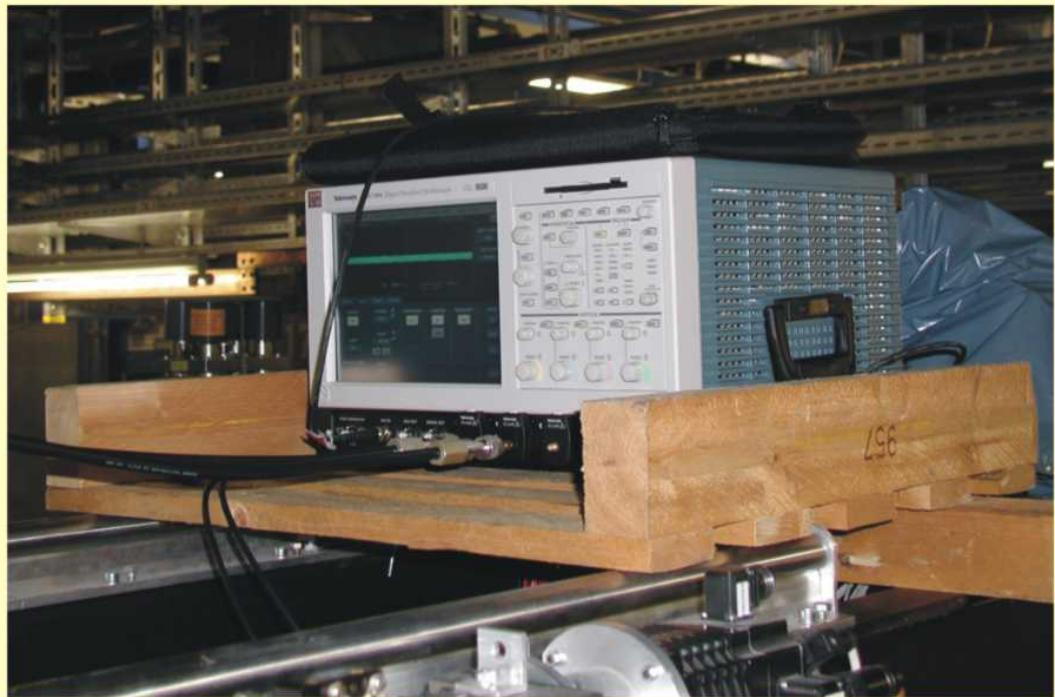
5 GHz bandwidth, 10 GHz sampling rate
