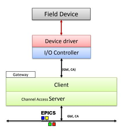
**I/O Controller (IOC)**: Any computing device (PC, SBC, micro-controller board, FPGA board etc.) able to manage the I/O of the field devices;
