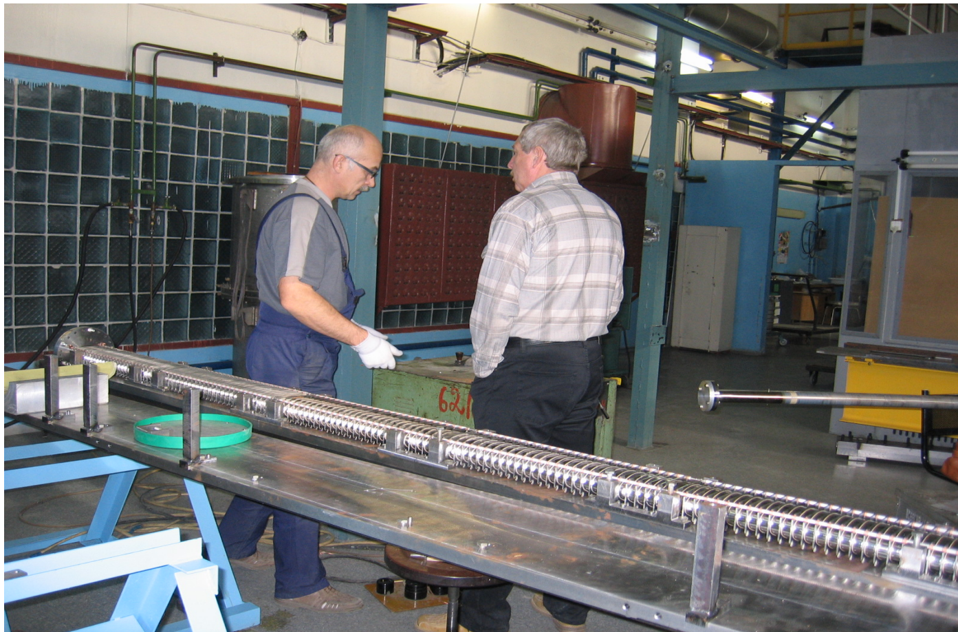
The SIS100 dipole chamber prototype under assembly
