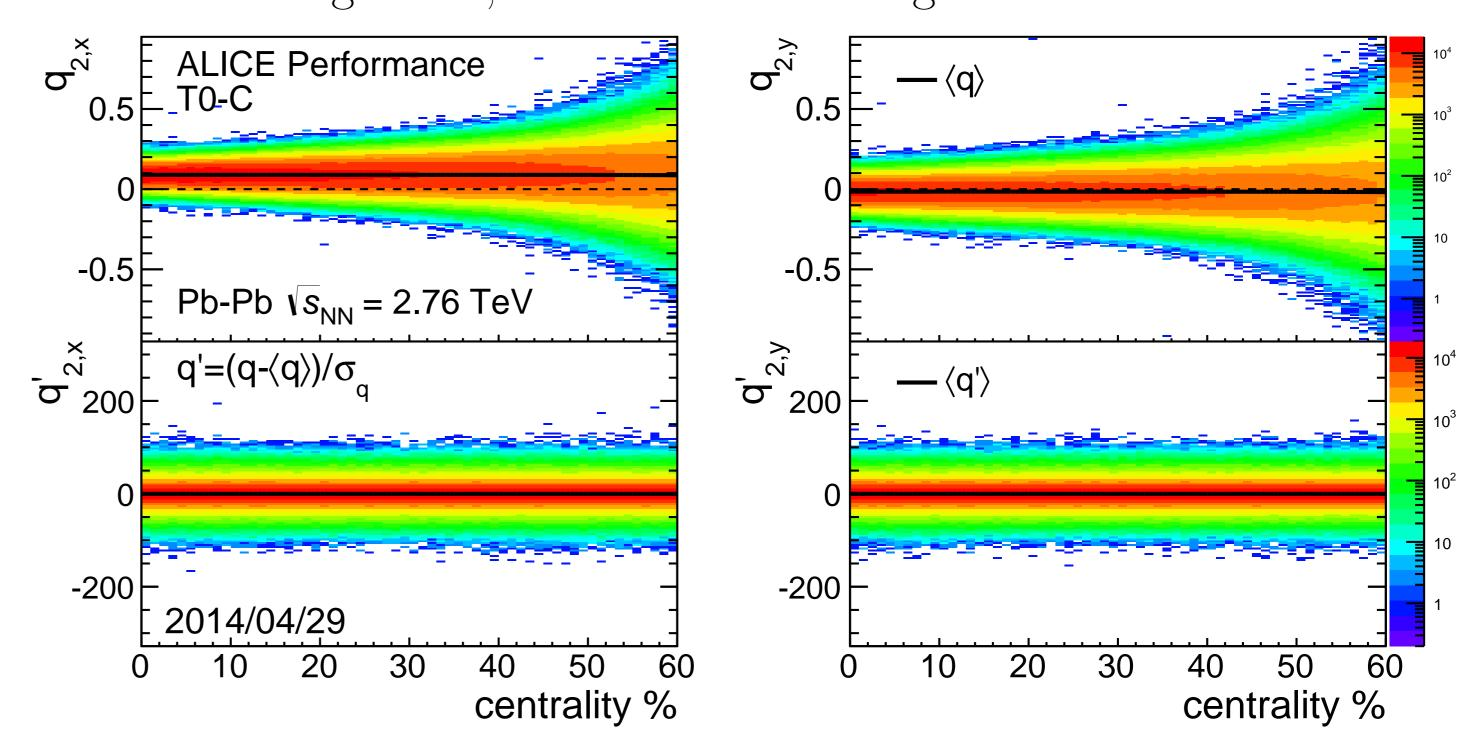
The figure illustrates the effect of q-vector recentering and width equalization for the T0-C measurement as a function of collision centrality for both q-vector components. The correction is applied as a function of event centrality and vertex position along the beam direction.
