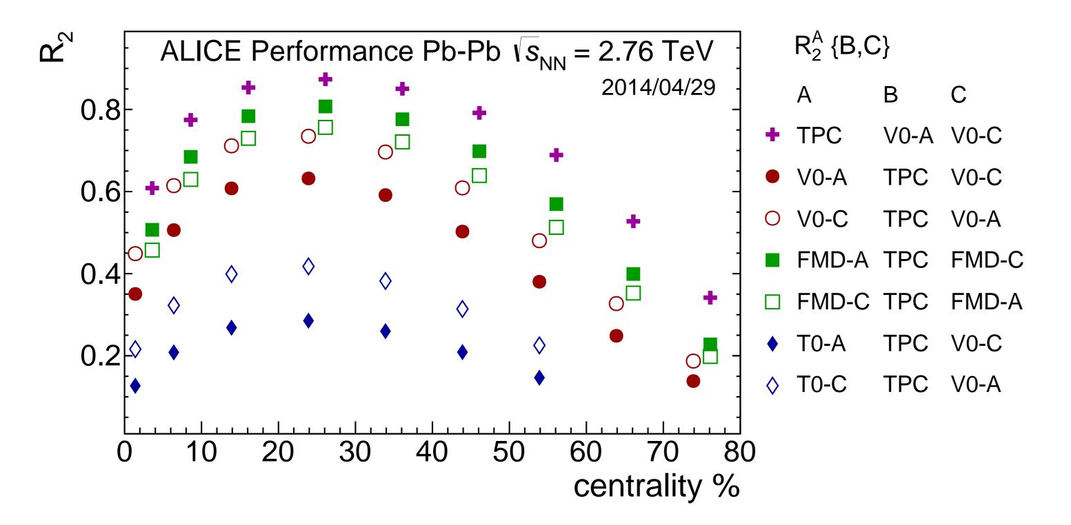
The T0, V0 and FMD detector resolution correction is shown separately for both sides of the interaction point. The event plane resolution correction is calculated with the 3-subevent method [1],
