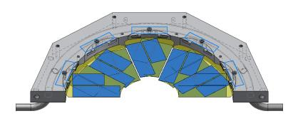
Requirement: Good thermal conducting contact between cooling pipe and aluminum
