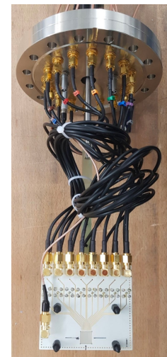
1cm x 1cm x 80 μm pcCVD diamond sensor
