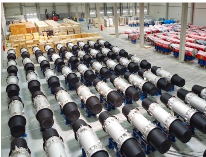
SIS100 dipoles ready for installation
