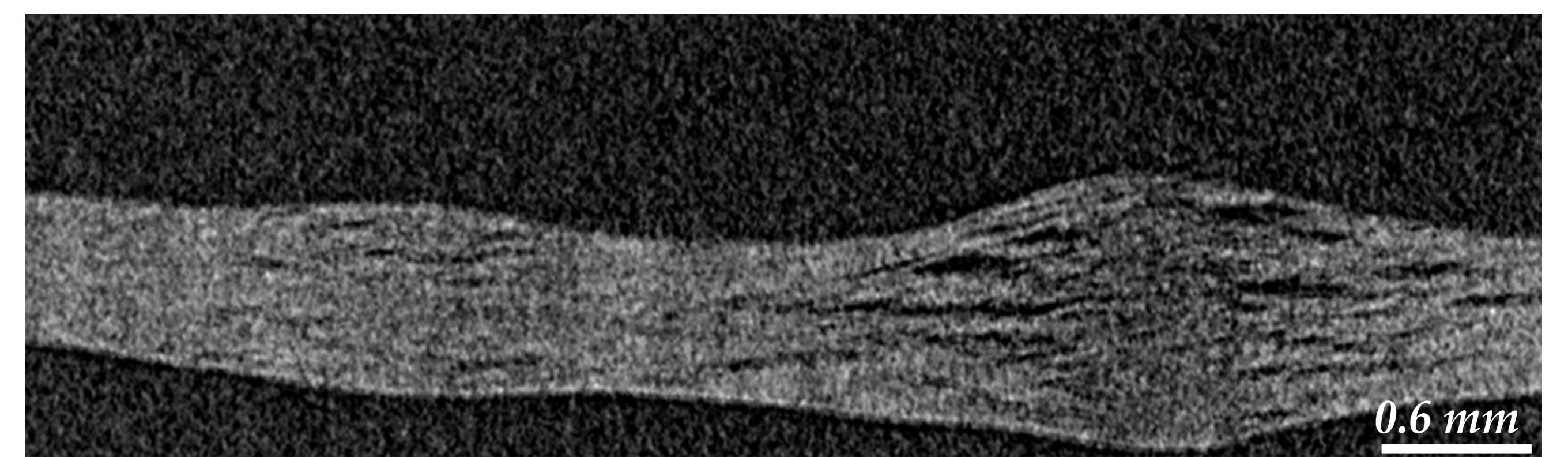
Figure 5: CT images of Sigraflex specimen after HiRadMat56 (top view and cross-sectional view)
