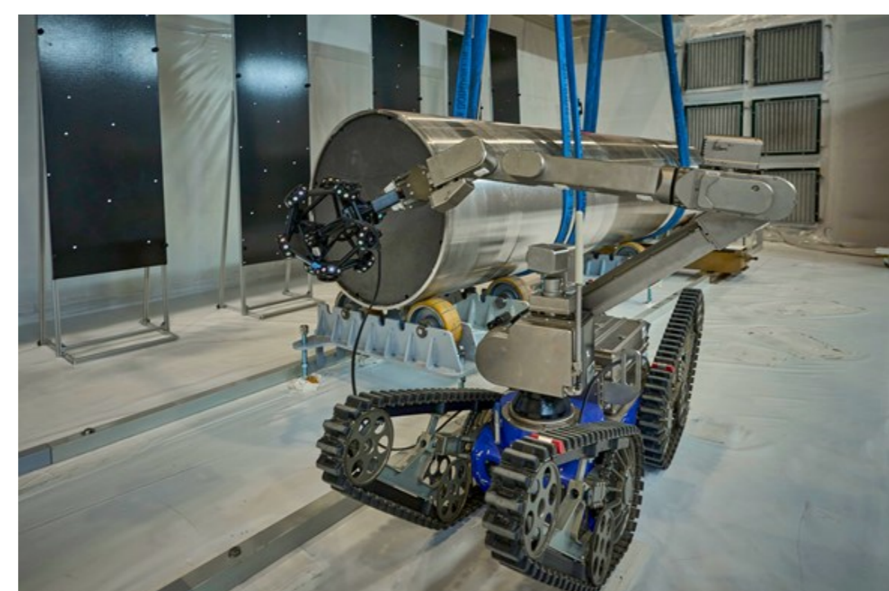
Figure 2: Portable 3D laser scanner mounted in a robot when the 318LN vessel was still on (images N. Solieri)
