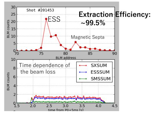
The extraction efficiency of 99.5% before the main power supply upgrade was well reproduced.
